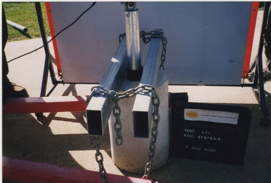
Figure 4.1.2. Test 471 Static pull force - wedge at 10mm. Maximum force 3,188N. (325kgf)
